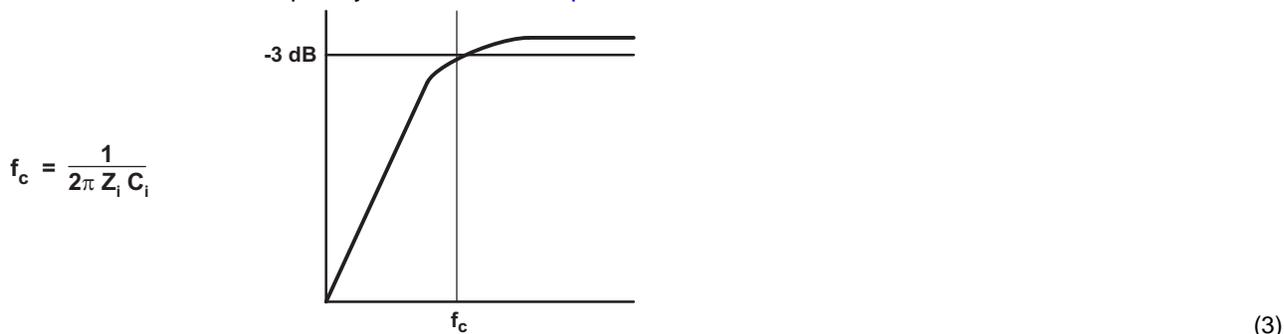
The value of  $C_i$  is important, as it directly affects the bass (low-frequency) performance of the circuit. Consider the example where  $Z_i$  is 60 kΩ and the specification calls for a flat bass response down to 20 Hz. [Equation 3](#) is reconfigured as [Equation 4](#).
