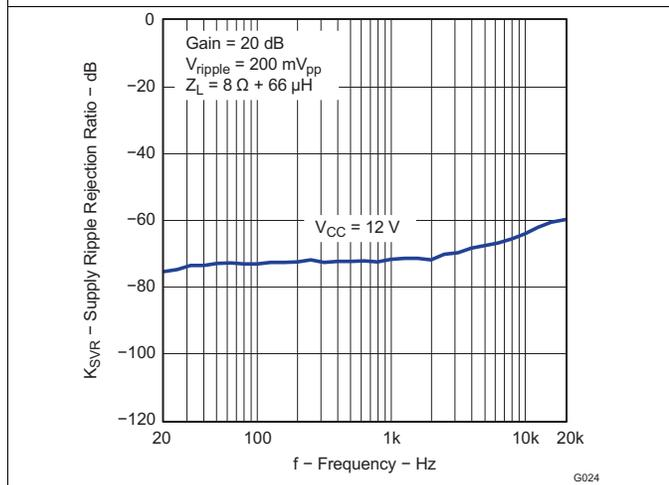
**Figure 27. Supply Ripple Rejection Ratio vs Frequency (BTL)**
