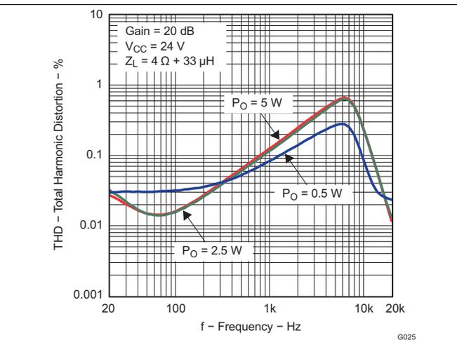
**Figure 28. Total Harmonic Distortion vs Frequency (PBTL)**
