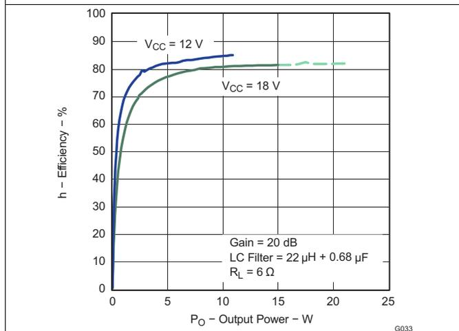
Figure 21. Efficiency vs Output Power (BTL With LC Filter)
