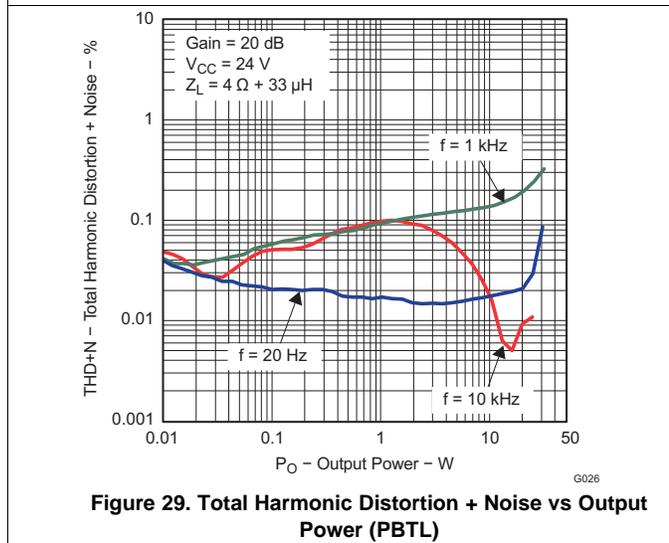
**Figure 29. Total Harmonic Distortion + Noise vs Output Power (PBTL)**
