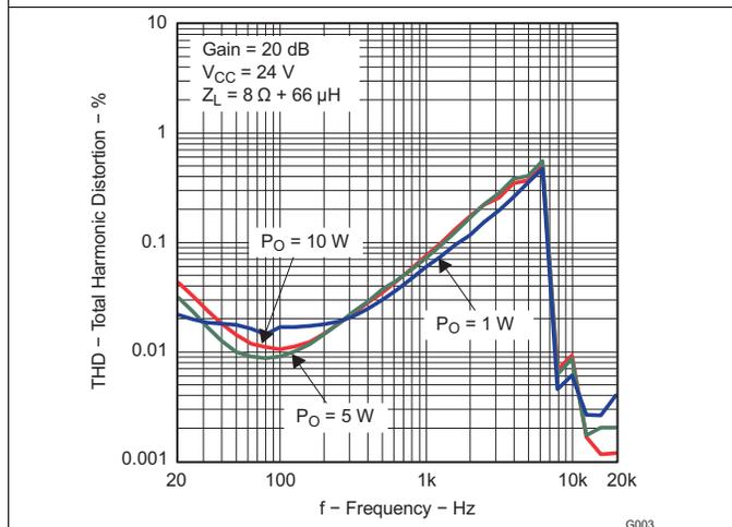
Figure 3. Total Harmonic Distortion vs Frequency (BTL)
