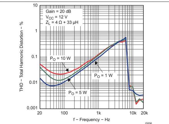
Figure 6. Total Harmonic Distortion vs Frequency (BTL)
