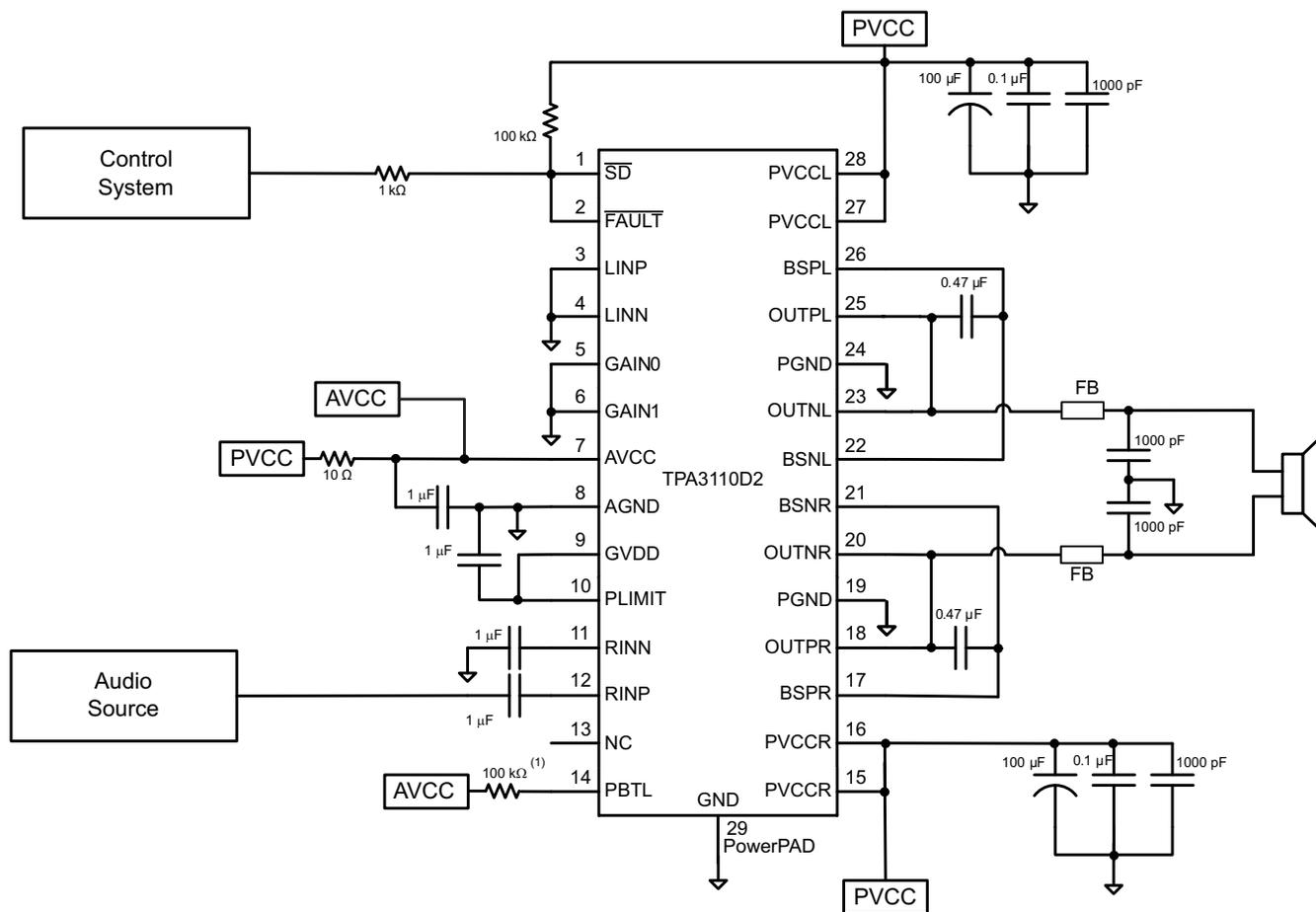
(1) 100 kΩ resistor is needed if the PVCC slew rate is more than 10 V/ms.
