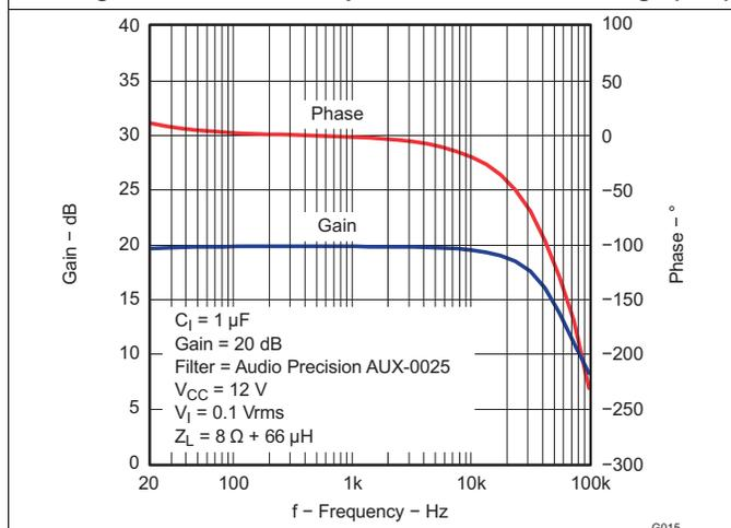
**Figure 15. Gain and Phase vs Frequency (BTL)**
