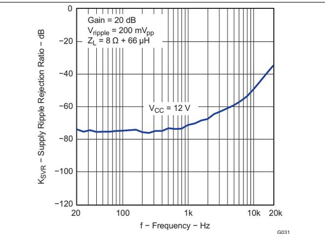
**Figure 34. Supply Ripple Rejection Ratio vs Frequency (PBTL)**
