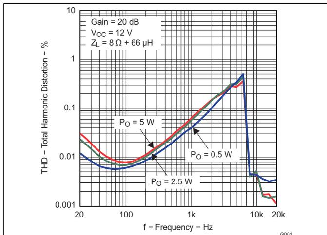
Figure 1. Total Harmonic Distortion vs Frequency (BTL)
