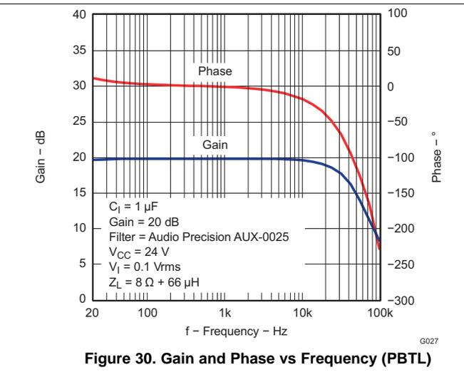
**Figure 30. Gain and Phase vs Frequency (PBTL)**
