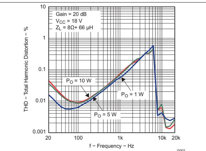
Figure 2. Total Harmonic Distortion vs Frequency (BTL)
