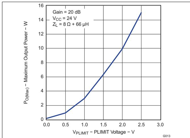
**Figure 13. Maximum Output Power vs PLIMIT Voltage (BTL)**
