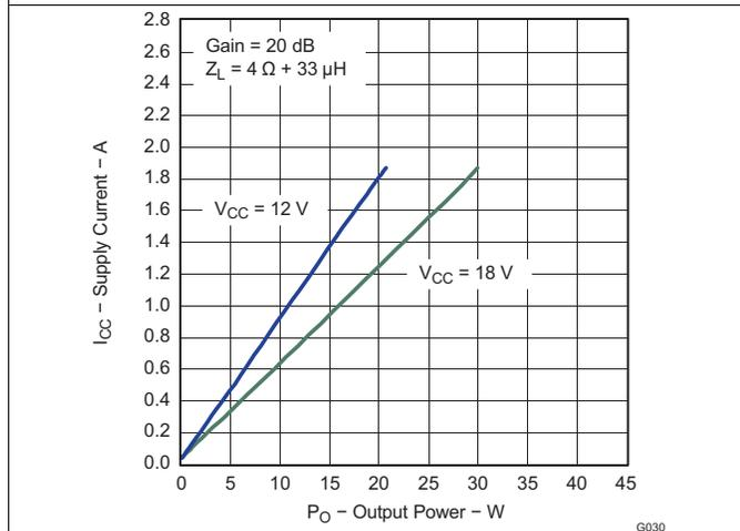
**Figure 33. Supply Current vs Output Power (PBTL)**
