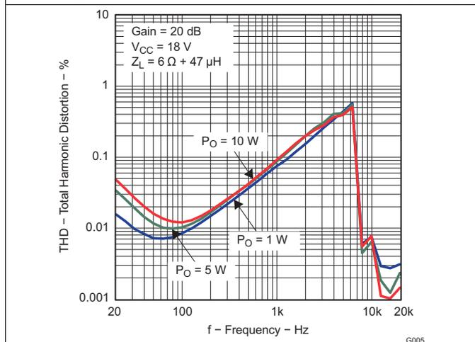
Figure 5. Total Harmonic Distortion vs Frequency (BTL)
