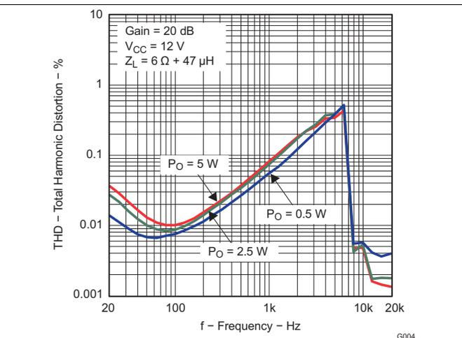
Figure 4. Total Harmonic Distortion vs Frequency (BTL)
