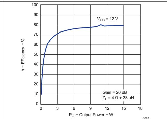
Figure 22. Efficiency vs Output Power (BTL)
